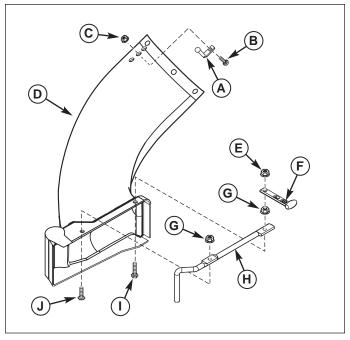
Figure 6. Lower Chute to Boot Installation
